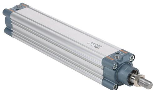
NITRA pneumatic cylinder, ISO 15552, 50mm bore, 20mm rod diameter, 250mm stroke, double acting, magnetic piston, front and rear adjustable cushions.
