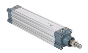
NITRA pneumatic cylinder, ISO 15552, 50mm bore, 20mm rod diameter, 200mm stroke, double acting, magnetic piston, front and rear adjustable cushions.
