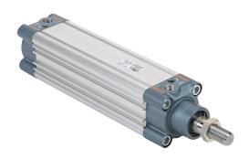
NITRA pneumatic cylinder, ISO 15552, 50mm bore, 20mm rod diameter, 150mm stroke, double acting, magnetic piston, front and rear adjustable cushions.
