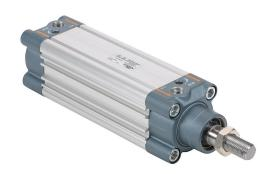
NITRA pneumatic cylinder, ISO 15552, 50mm bore, 20mm rod diameter, 100mm stroke, double acting, magnetic piston, front and rear adjustable cushions.
