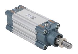
NITRA pneumatic cylinder, ISO 15552, 50mm bore, 20mm rod diameter, 50mm stroke, double acting, magnetic piston, front and rear adjustable cushions.
