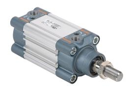
NITRA pneumatic cylinder, ISO 15552, 50mm bore, 20mm rod diameter, 25mm stroke, double acting, magnetic piston, front and rear adjustable cushions.
