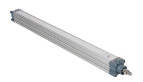
NITRA pneumatic cylinder, ISO 15552, 40mm bore, 16mm rod diameter, 600mm stroke, double acting, magnetic piston, front and rear adjustable cushions.
