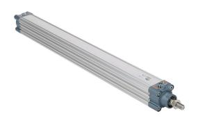
NITRA pneumatic cylinder, ISO 15552, 40mm bore, 16mm rod diameter, 500mm stroke, double acting, magnetic piston, front and rear adjustable cushions.
