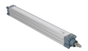
NITRA pneumatic cylinder, ISO 15552, 40mm bore, 16mm rod diameter, 400mm stroke, double acting, magnetic piston, front and rear adjustable cushions.
