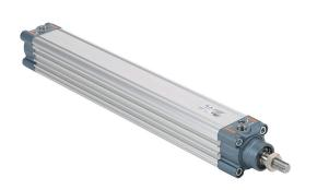
NITRA pneumatic cylinder, ISO 15552, 40mm bore, 16mm rod diameter, 300mm stroke, double acting, magnetic piston, front and rear adjustable cushions.
