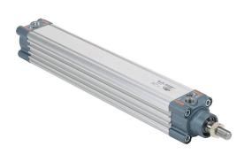
NITRA pneumatic cylinder, ISO 15552, 40mm bore, 16mm rod diameter, 250mm stroke, double acting, magnetic piston, front and rear adjustable cushions.
