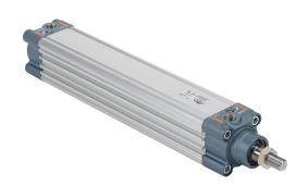
NITRA pneumatic cylinder, ISO 15552, 40mm bore, 16mm rod diameter, 200mm stroke, double acting, magnetic piston, front and rear adjustable cushions.
