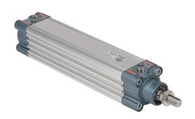
NITRA pneumatic cylinder, ISO 15552, 40mm bore, 16mm rod diameter, 150mm stroke, double acting, magnetic piston, front and rear adjustable cushions.
