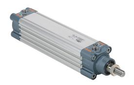
NITRA pneumatic cylinder, ISO 15552, 40mm bore, 16mm rod diameter, 125mm stroke, double acting, magnetic piston, front and rear adjustable cushions.
