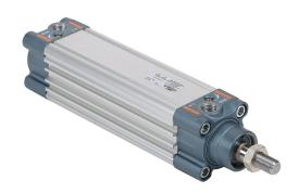
NITRA pneumatic cylinder, ISO 15552, 40mm bore, 16mm rod diameter, 100mm stroke, double acting, magnetic piston, front and rear adjustable cushions.
