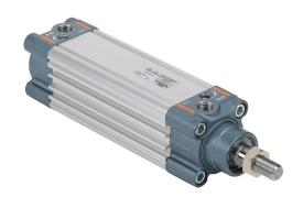
NITRA pneumatic cylinder, ISO 15552, 40mm bore, 16mm rod diameter, 75mm stroke, double acting, magnetic piston, front and rear adjustable cushions.
