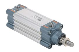
NITRA pneumatic cylinder, ISO 15552, 40mm bore, 16mm rod diameter, 50mm stroke, double acting, magnetic piston, front and rear adjustable cushions.
