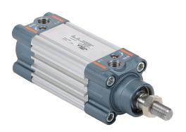
NITRA pneumatic cylinder, ISO 15552, 40mm bore, 16mm rod diameter, 25mm stroke, double acting, magnetic piston, front and rear adjustable cushions.
