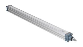
NITRA pneumatic cylinder, ISO 15552, 32mm bore, 12mm rod diameter, 600mm stroke, double acting, magnetic piston, front and rear adjustable cushions.
