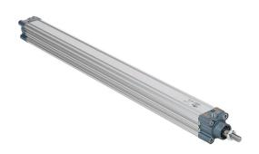
NITRA pneumatic cylinder, ISO 15552, 32mm bore, 12mm rod diameter, 500mm stroke, double acting, magnetic piston, front and rear adjustable cushions.
