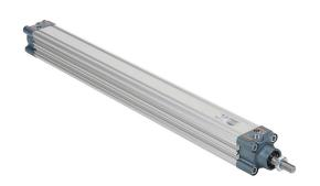
NITRA pneumatic cylinder, ISO 15552, 32mm bore, 12mm rod diameter, 400mm stroke, double acting, magnetic piston, front and rear adjustable cushions.
