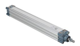
NITRA pneumatic cylinder, ISO 15552, 32mm bore, 12mm rod diameter, 300mm stroke, double acting, magnetic piston, front and rear adjustable cushions.
