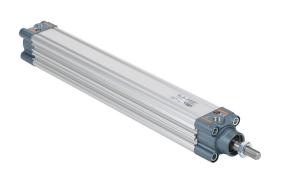
NITRA pneumatic cylinder, ISO 15552, 32mm bore, 12mm rod diameter, 250mm stroke, double acting, magnetic piston, front and rear adjustable cushions.
