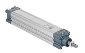
NITRA pneumatic cylinder, ISO 15552, 32mm bore, 12mm rod diameter, 150mm stroke, double acting, magnetic piston, front and rear adjustable cushions.
