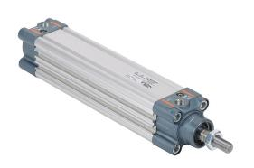
NITRA pneumatic cylinder, ISO 15552, 32mm bore, 12mm rod diameter, 125mm stroke, double acting, magnetic piston, front and rear adjustable cushions.
