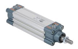
NITRA pneumatic cylinder, ISO 15552, 32mm bore, 12mm rod diameter, 75mm stroke, double acting, magnetic piston, front and rear adjustable cushions.
