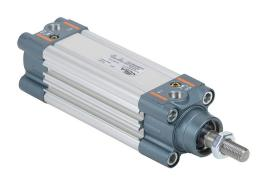
NITRA pneumatic cylinder, ISO 15552, 32mm bore, 12mm rod diameter, 50mm stroke, double acting, magnetic piston, front and rear adjustable cushions.
