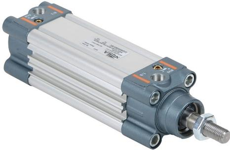
NITRA pneumatic cylinder, ISO 15552, 32mm bore, 12mm rod diameter, 50mm stroke, double acting, magnetic piston, front and rear adjustable cushions.
