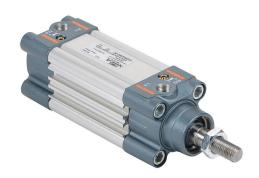
NITRA pneumatic cylinder, ISO 15552, 32mm bore, 12mm rod diameter, 25mm stroke, double acting, magnetic piston, front and rear adjustable cushions.
