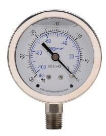
ProSense mechanical pressure gauge, 2.5in diameter, -30 to 0in Hg vacuum/-100 to 0 kPa, stainless steel liquid filled case, stainless steel wetted parts, 1/4in male NPT process connection, lower mount.
