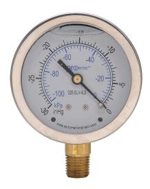
ProSense mechanical pressure gauge, 2.5in diameter, -30 to 0in Hg vacuum/-100 to 0 kPa, stainless steel liquid filled case, brass wetted parts, 1/4in male NPT process connection, lower mount.
