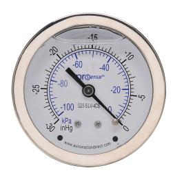
ProSense mechanical pressure gauge, 2.5in diameter, -30 to 0in Hg vacuum/-100 to 0 kPa, stainless steel liquid filled case, stainless steel wetted parts, 1/4in male NPT process connection, center back mount.
