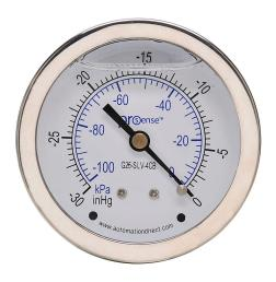
ProSense mechanical pressure gauge, 2.5in diameter, -30 to 0in Hg vacuum/-100 to 0 kPa, stainless steel liquid filled case, brass wetted parts, 1/4in male NPT process connection, center back mount.
