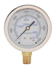
ProSense mechanical pressure gauge, 2.5in diameter, 0 to 6000 psig/0 to 42000 kPa, stainless steel liquid filled case, brass wetted parts, 1/4in male NPT process connection, lower mount.
