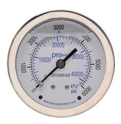
ProSense mechanical pressure gauge, 2.5in diameter, 0 to 6000 psig/0 to 42000 kPa, stainless steel liquid filled case, brass wetted parts, 1/4in male NPT process connection, center back mount.
