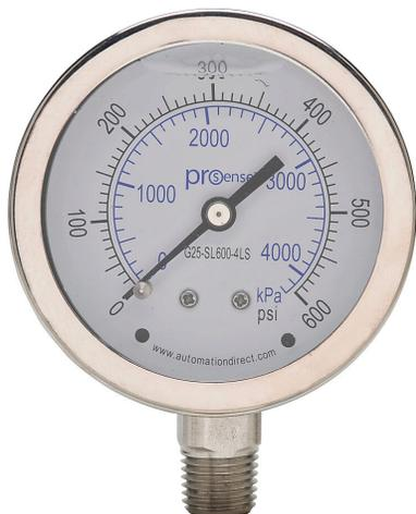
ProSense mechanical pressure gauge, 2.5in diameter, 0 to 600 psig/0 to 4200 kPa, stainless steel liquid filled case, stainless steel wetted parts, 1/4in male NPT process connection, lower mount.
