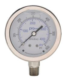
ProSense mechanical pressure gauge, 2.5in diameter, 0 to 600 psig/0 to 4200 kPa, stainless steel liquid filled case, stainless steel wetted parts, 1/4in male NPT process connection, lower mount.
