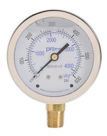
ProSense mechanical pressure gauge, 2.5in diameter, 0 to 600 psig/0 to 4200 kPa, stainless steel liquid filled case, brass wetted parts, 1/4in male NPT process connection, lower mount.
