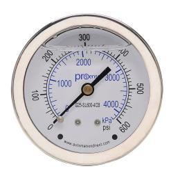
ProSense mechanical pressure gauge, 2.5in diameter, 0 to 600 psig/0 to 4200 kPa, stainless steel liquid filled case, brass wetted parts, 1/4in male NPT process connection, center back mount.
