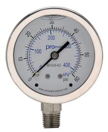
ProSense mechanical pressure gauge, 2.5in diameter, 0 to 60 psig/0 to 420 kPa, stainless steel liquid filled case, stainless steel wetted parts, 1/4in male NPT process connection, lower mount.
