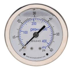
ProSense mechanical pressure gauge, 2.5in diameter, 0 to 60 psig/0 to 420 kPa, stainless steel liquid filled case, stainless steel wetted parts, 1/4in male NPT process connection, center back mount.
