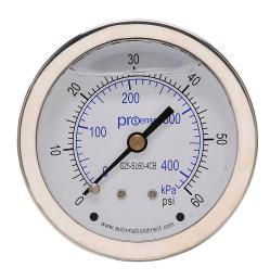
ProSense mechanical pressure gauge, 2.5in diameter, 0 to 60 psig/0 to 420 kPa, stainless steel liquid filled case, brass wetted parts, 1/4in male NPT process connection, center back mount.
