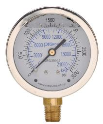
ProSense mechanical pressure gauge, 2.5in diameter, 0 to 3000 psig/0 to 21000 kPa, stainless steel liquid filled case, brass wetted parts, 1/4in male NPT process connection, lower mount.
