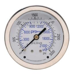
ProSense mechanical pressure gauge, 2.5in diameter, 0 to 3000 psig/0 to 21000 kPa, stainless steel liquid filled case, brass wetted parts, 1/4in male NPT process connection, center back mount.
