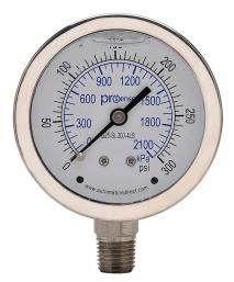
ProSense mechanical pressure gauge, 2.5in diameter, 0 to 300 psig/0 to 2100 kPa, stainless steel liquid filled case, stainless steel wetted parts, 1/4in male NPT process connection, lower mount.
