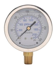
ProSense mechanical pressure gauge, 2.5in diameter, 0 to 300 psig/0 to 2100 kPa, stainless steel liquid filled case, brass wetted parts, 1/4in male NPT process connection, lower mount.
