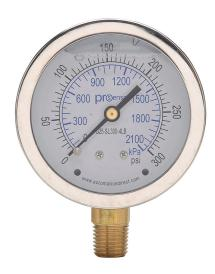
ProSense mechanical pressure gauge, 2.5in diameter, 0 to 300 psig/0 to 2100 kPa, stainless steel liquid filled case, brass wetted parts, 1/4in male NPT process connection, lower mount.
