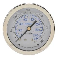
ProSense mechanical pressure gauge, 2.5in diameter, 0 to 300 psig/0 to 2100 kPa, stainless steel liquid filled case, brass wetted parts, 1/4in male NPT process connection, center back mount.
