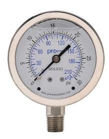
ProSense mechanical pressure gauge, 2.5in diameter, 0 to 30 psig/0 to 210 kPa, stainless steel liquid filled case, stainless steel wetted parts, 1/4in male NPT process connection, lower mount.
