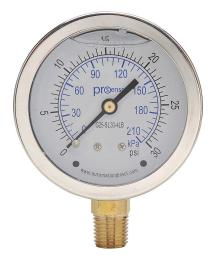
ProSense mechanical pressure gauge, 2.5in diameter, 0 to 30 psig/0 to 210 kPa, stainless steel liquid filled case, brass wetted parts, 1/4in male NPT process connection, lower mount.
