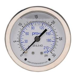
ProSense mechanical pressure gauge, 2.5in diameter, 0 to 30 psig/0 to 210 kPa, stainless steel liquid filled case, stainless steel wetted parts, 1/4in male NPT process connection, center back mount.
