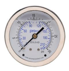
ProSense mechanical pressure gauge, 2.5in diameter, 0 to 30 psig/0 to 210 kPa, stainless steel liquid filled case, brass wetted parts, 1/4in male NPT process connection, center back mount.
