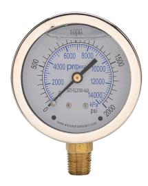
ProSense mechanical pressure gauge, 2.5in diameter, 0 to 2000 psig/0 to 14000 kPa, stainless steel liquid filled case, brass wetted parts, 1/4in male NPT process connection, lower mount.
